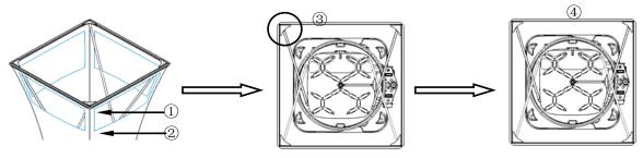
Use the angled corners ① and the stitching ② as a guide to ensure the hood is straight. If the fabric hood is twisted it will not assemble correctly.
