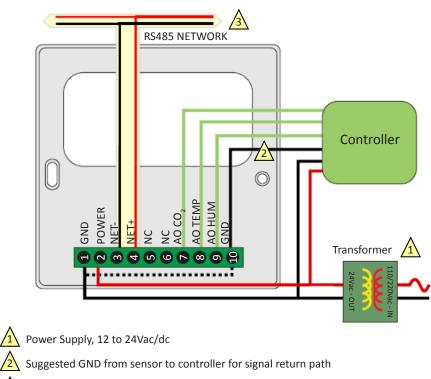
RS485 Net, 18ga twisted pair typical, optional ground & shield
