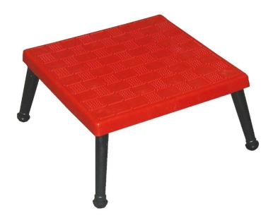
Insulating platform with anti-slip surface made by resin reinforced by fiberglass. Dimensions 500x500x4 mm.
