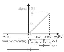
Note: In an unidirectional design, the switching output OC1 is used as a flow indicator by default (configurable). It indicates a flow greater than 0 m/s by blocking and switches through in case flow is smaller or equal 0 m/s. The arrows in the figure of the switching outputs signify that the threshold value is configurable.
