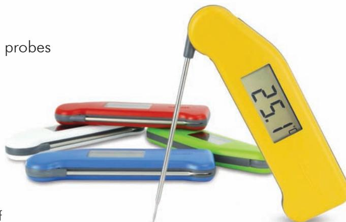
The SuperFast Thermapen 3 thermometer incorporates a large digital display with a precise read-out of temperature over the range of -49.9 to 299.9 °C with a 0.1 °C resolution and an accuracy of  $\pm 0.4$  °C.
