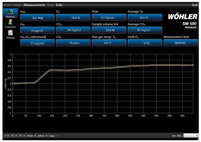
All measurement data and online readings can be transferred to a computer by USB connection. The Wöhler SM 500 computer software package allows extensive data analysis and display.
