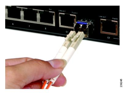
STEP 4 Connect the other end of the cable to an SFP module to verify that the fiber connection is complete.
