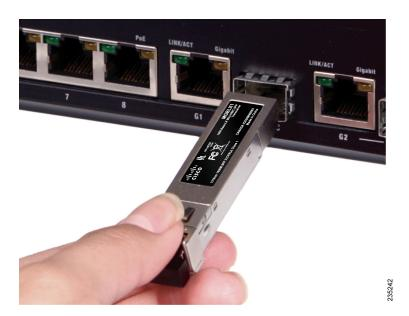
STEP 2 Remove the mini-GBIC SFP module's rubber port cap.
