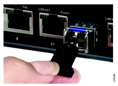
**STEP 3** Connect the fiber cable's LC connector to the mini-GBIC SFP module's port.
