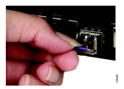
STEP 3 Remove the mini-GBIC SFP module.
