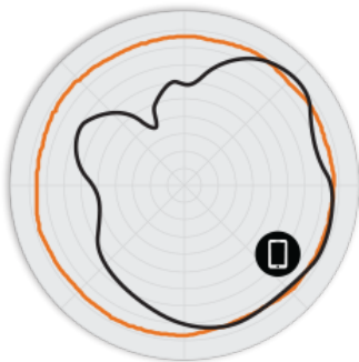
Figure 2. R610 2.4GHz Azimuth Antenna Patterns
