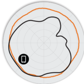
Figure 3. R610 5GHz Azimuth Antenna Patterns
