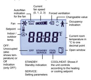
It is possible to set different parameter values in a parameter menu in the display, using the buttons on the controller. You change parameter values with the INCREASE and DECREASE buttons and confirm changes with the Occupancy button.
