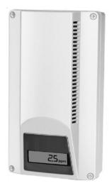
The model DCO-S3 is a digital ventilation controller specifically designed to monitor carbon monoxide and temperature in the enclosed or semi-enclosed car parks and to regulate the environment according to these two parameters. DCO-S3 is designed for easy installation and minimum maintenance during operation. It can be operated in stand-alone mode, as well as connected to larger building management systems.
