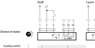
Auxiliary switch Connected with conductors S1, S2 and S3 (only model RDAB10-230S)
