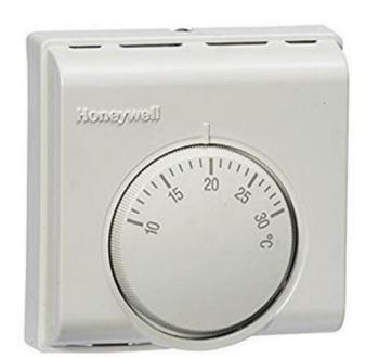
T6360 Thermostat are range of thermostats that are designed to provide automatic ON/OFF control for gas valves, circulation pumps, relays and zone valves in heating, cooling. Thermostat are available, in a wide range of feature combinations. These thermostat have dual diaphragm sensing element which ensures close temperature control for all loads and applications.
