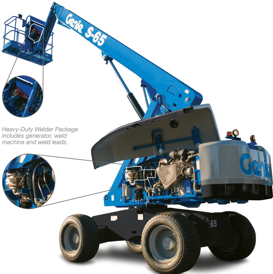
*Heavy-Duty Welder Package includes generator, weld machine and weld leads.*
