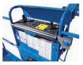
as possible to operators, featuring a pressure sensitive horizontal bar that is fitted at around waist height below the boom lift's control panel. The OPA system interrupts all boom functions when excessive pressure is applied to the sensing bar. The system also features a reset button that can be pressed if the system is inadvertently activated.
