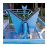
platform deck. The pipe cradle assembly mounts easily to the platform guardrails with U-bolts and rests on the floor of the platform when installed.
