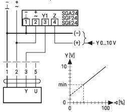
Control with 4...20 mA via external resistor
