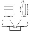
FCAW & GMAW Applied ROOT GAP 3-5mm steel structure of the ocean, shipbuilding, plant etc.
