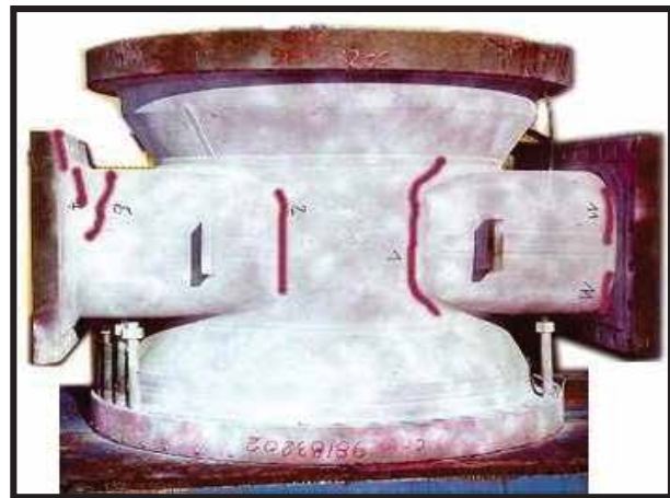
“ Valve Dye Penetration Inspection ”
