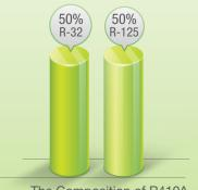
The Composition of R410A R-32: CH<sub>2</sub>F<sub>2</sub>; R-125: C<sub>2</sub>HF<sub>5</sub>
