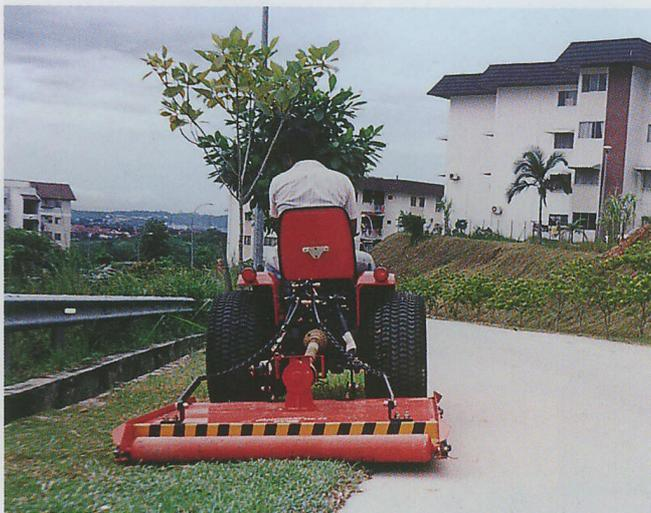
The ideal cutting height very much depends on the usage of the turf. Only one third of the length of a leaf should be cut off, so as to avoid "shocking" the grass plant's natural balance between root-net and leaf surface area. If the turf is extensively used, it should be allowed to develop strong grass leaves, i.e. cut often, but not too short. HOWARD rotaslashers have swing-back aero-dynamic blades, which lift the grass prior to cutting.
