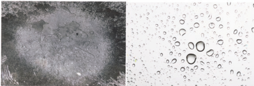
Surface after treated with HCA-120 when contacted with water
