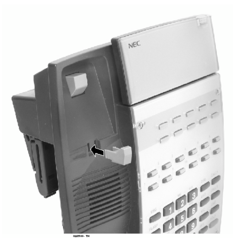
Figure 4-46: INSTALLING THE HOOKSWITCH HANGER
