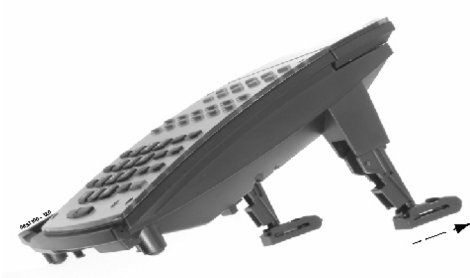
Figure 4-42: EXTENDING THE LEGS - POSITION 3
