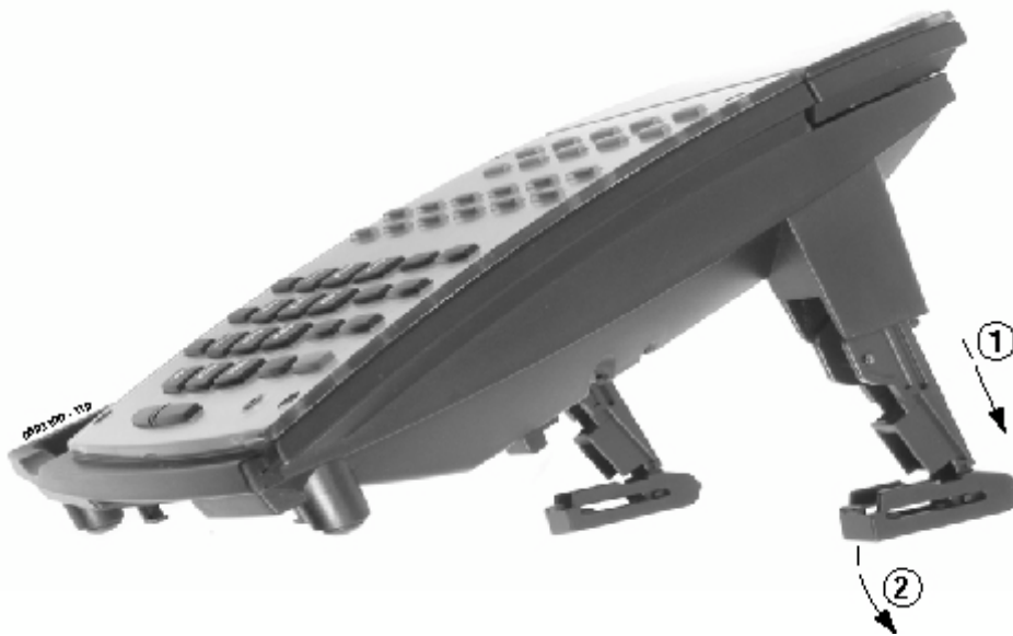
Figure 4-41: EXPANDING THE LEG HEIGHT - POSITION 3
