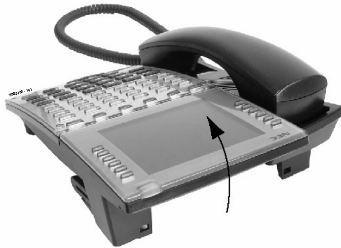
Figure 3-3: LIFTING THE LCD DISPLAY
