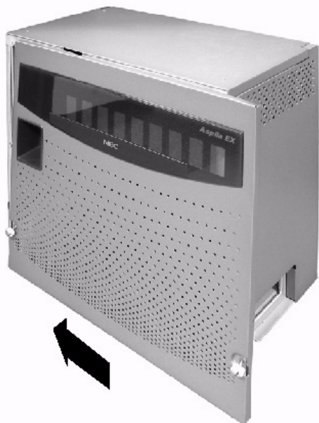
Figure 1-37: RE-INSTALLING THE FRONT COVER
