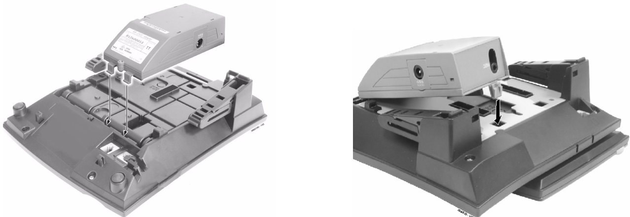
Figure 4-32: POSITIONING THE ADAPTER
