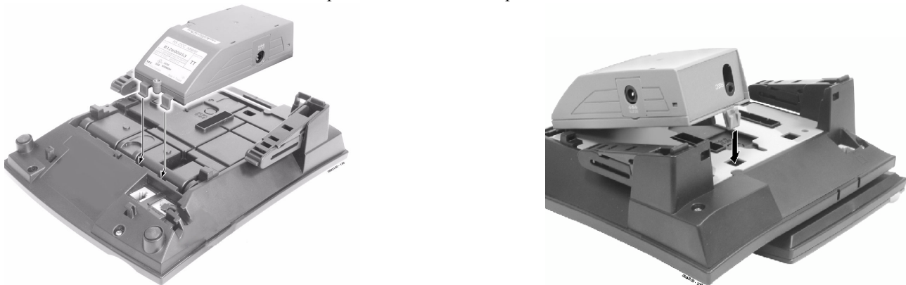
Figure 4-30: POSITIONING THE ADAPTER
