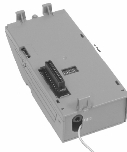
Figure 4-22: RUNNING THE CABLE TO THE ADA
