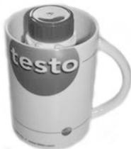
2. Heat water in a container (e.g. a cup) to approx. 50 °C. Place closed reference oil bottle in the water bath for approx. 10 min (maximum water level to lower edge of sealing cap). Then briefly shake the closed reference oil bottle, for better heat distribution in the bottle.
