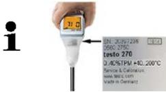
The last two figures of the instrument's serial number are automatically set as the PIN (see sticker on the instrument).
