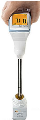
5. Immerse sensor in reference oil. Adhere to the immersion depth!
