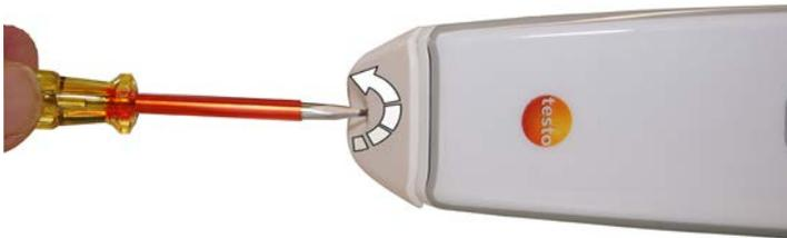
1. Undo the screw on the battery compartment.
