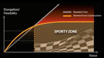
In the sporty zone, the Xtreme-Force ply material causes MC6 to be more rigid which provides a direct feedback to the driver.A conventional ply material would be flexing much more which reduces the feedback in cornering and steering at high speeds.
