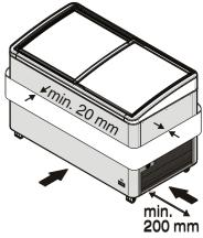
Do not place any objects immediately next to the outer housing of the appliance. There must be a gap of at least 20 mm all round in order to ensure adequate beat
