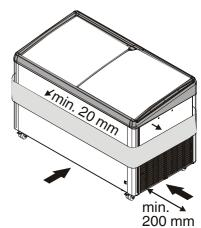
Standard EN 378 specifies that the room in which you install your appliance must have a volume of 1 m³ per 8 g of R 290a/ R 600a refrigerant used in the appliance, so as to avoid the formation of inflammable gas/air mixtures in the room where the appliance is located in the event of a leak in the refrigerant circuit. The quantity of refrigerant used in your appliance is indicated on the type plate
