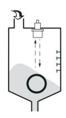
The transducer should not be mounted too close to the tank wall, the build-up on the tank wall cause false echoes.
