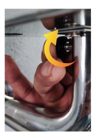
14. Turn the screw until it is tight to make sure the METS raks is lock
