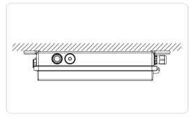
Fix the fixture to the ceiling through the two mounting holes on the fixture.
