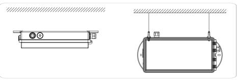
First, connect the two pendant strings with the fixture. Then fix it on the ceiling.
