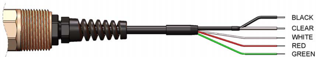
Figure 3.4: pH sensor hook-up – No integral pre-amplifier
