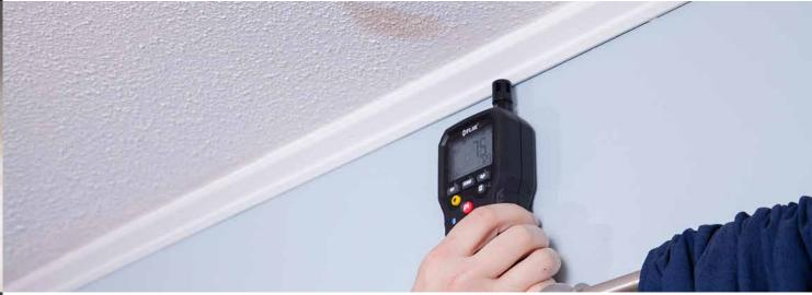
Everything you need in a meter for moisture remediation or HVAC: Bluetooth<sup>®</sup> METERLiNK capability, a pinless moisture sensor and pin probe, a temperature and relative humidity sensor, and an IR thermometer
