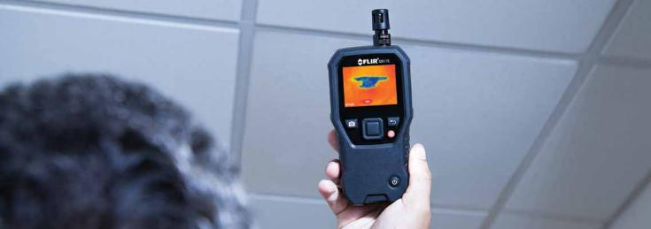
Featuring IGM technology powered by a built-in thermal imaging sensor, the MR176 and MR160 can visually guide you to the precise spot that moisture may be hiding
