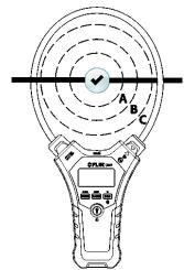
Fig. 7-1 Positioning Conductor in Clamp Jaw center
