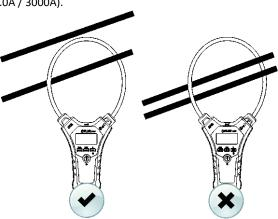
Fig. 5-2 Correct (left) and Incorrect (right) **Conductor Clamping**
