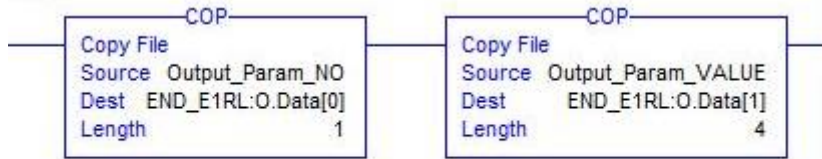
Figure 46: Controller tags: Parameter number and value and their destination registers in the device
