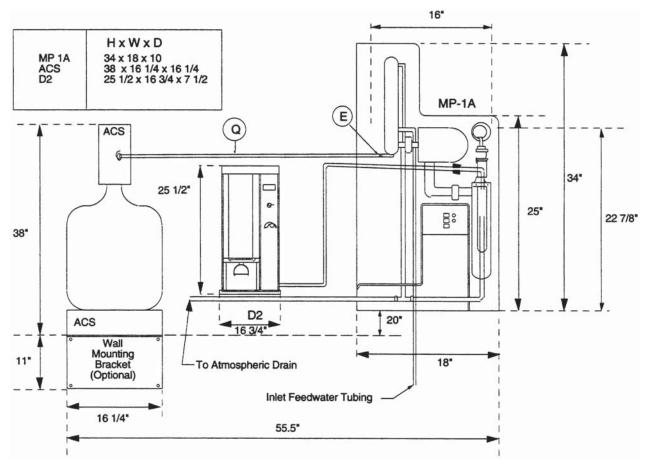
Figure 9-2. Complete System Layout (not to scale)
