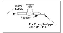
Figure 6-4. Shut-off Valve
