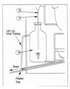
Figure 9-1. Storage Bottle Installation
