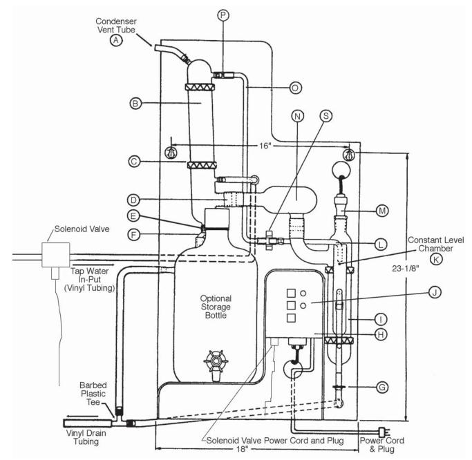
Figure 10-1. Still Components and Connections
