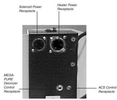
Figure 7-1. Control Bottom Connections
