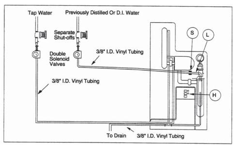
Figure 8-4. In-House Treated Feed
