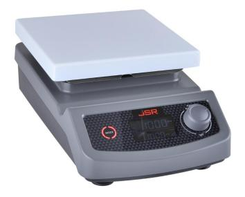
JSHS-18D Digital hotplate Stirrer utilize the most advanced Digital Fuzzy Control technology of temperature, stirring speed and time. Control temperature range max. 400 °C in 0.1 °C display resolution, stirring speed range from 80 to 1,500 rpm, timer set to 99 hr 59 min. Durable and rugged aluminum casting body and chemical resistant ceramic coated top plate.
