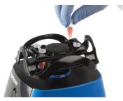
1.5/2 mL microfuge tubes x 4 (vertically mounted)
