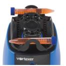
15 mL conical tubes x 2 (horizontally mounted)
