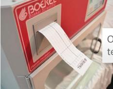
On-Board Thermal Printer for quick and easy temperature record keeping
