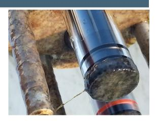
The TurbiTechw<sup>2</sup> LS Sensor is designed to monitor the levels of suspended solids or turbidity typically found in final effluent from municipal and industrial wastewater treatment plants. It is also great at monitoring solids in the intake to both effluent and drinking water treatment processes.
