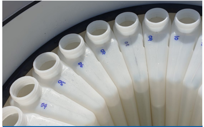
Wastewater samples collected using a composite sampling program by YSI ProSample.
