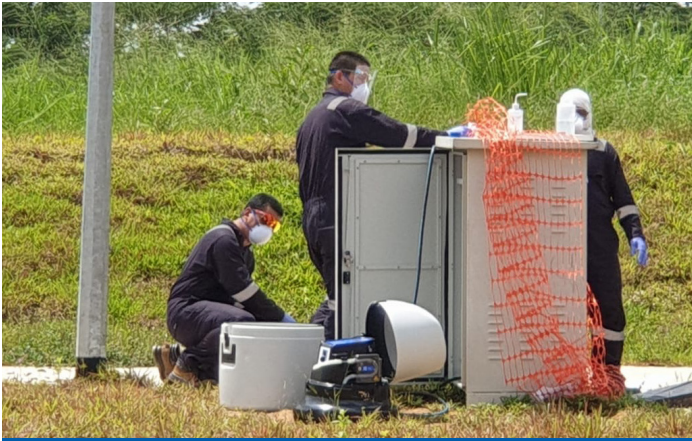
Wastewater samples are collected by a field team and sent to a laboratory for COVID RNA testing.
