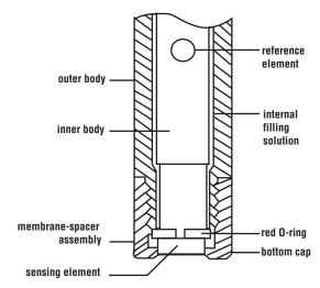
Figure 4 Construction Of The Carbon Dixoide Electrode
