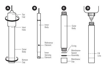
Figure 1 Electrode Assembly and Preparation
