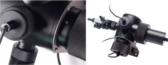
The TurbiTechw<sup>2</sup> LR Sensor has been specifically designed to monitor final treated, potable and filter water. The sensor is extremely sensitive and is capable of discriminating changes in Turbidity of less than 0.1 FTU. The 90° light scatter monitoring technique makes the sensor sensitive to a wide range of particle sizes, from colloidal material throughto larger particles, raw water and the large mineral particles sometimes found in distribution samples.
