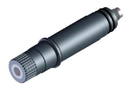
The WaterTechw² pH8000 Sensor has been designed to provide highly reliable pH and Temperature measurements. The sensor uses a flat surfaced electrode which includes an extended reference path, these features combine to provide an extremely robust pH measurement, suitable for use in surface water, wastewater and drinking water applications.
