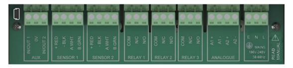
The maximum size wire that can be terminated is 2.5mm<sup>2</sup> CSA. All the connections are via removable Plug/Socket terminals. To disengage the terminal strip, simply pull down to release.
