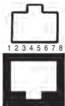
RJ45 SOCKET/PLUG PIN DIAGRAM
