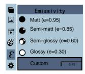
As shown in the figure, press " $^{\circ}$ " (MENU", key to enter the main menu and select " $^{\circ}$ " (emissivity) option and press " $^{\bullet}$ " key to enter the emissivity lists.
