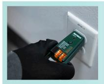
Rugged and affordable receptacle testers with convenient features like ergonomic pull bar and legend on both sides. These testers stand out due to their reliability, ease of use, and affordability. They are especially designed for detecting various wiring faults in electrical outlets. The ET11 comes with the ability to confirm the operation of GFCI circuits.
