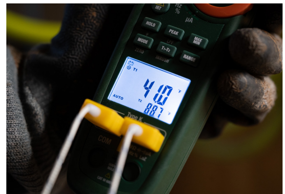
Dual Type K thermometer for taking differential temperature readings needed for superheat measurements.
