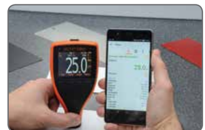
USB and Bluetooth® data output to iPhone 2 or Android™ devices
