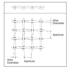
Flattop weave is used for screening large and middle-size particles. The surface of the mesh is designed to be flat and smooth.
