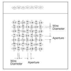
Flat weave mesh is basic as each wire crosses vertically to keep the aperture squares stable in the screen. This standard cross enables accurate and effective screening.
