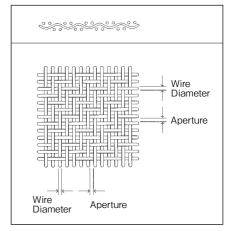
Twill weave mesh is structured by crossing two parallel wires with each other in one uneven pattern. The mesh is woven using thick wires and is good for screening small particles.
