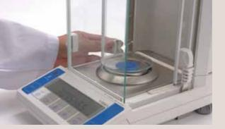
VIBRA LF series is equipped with "cross-over sliding" windshield which enables the user to open the right-side door by left-side knob, vice versa. The user can handle the weighing sample with right hand while he/she operates the door with left hand. It makes weighing operation in lab routines less time-consuming.
