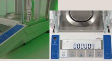
The regular calibration is highly important to assure the reliable weighing result. "Se-CAL" function in VIBRA LF series performs automatic calibration. When elapsed time or temperature shift leach to defined value, "Se-CAL" carries out the calibration fully automatically. The calibration record can be stored in the balance and output later on.
