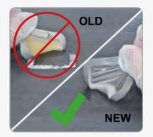
Elcometer 135C Bresle Test Patches are easy to peel off after a test, leaving no foam on the substrate, causing less damage as no need to scrape off residue.
